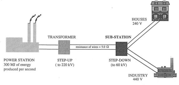
a) When the power is transmitted over large distances, thick inexpensive wires are used to transmit the energy at high voltages. Why are **thick** wires used?
