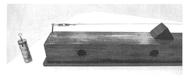
Students conducted an experiment, using a sonometer. Increasing the mass that is suspended from one end of the wire varies the tension in the wire. The lowest frequency of the vibrating wire is measured (in Hz) using an appropriate app on a smartphone, as shown in the photograph below.
